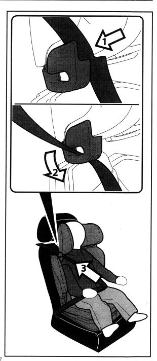
**4.** To remove the belt, slide it out of the router slot (1) and then between the router and the headrest (2) until it is completely removed.
