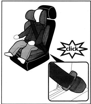
**3.** Thread the belt through the router placed on the headrest: thread the belt between the router and the headrest (1) until it slides completely into the router slot (2).
