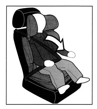
**2.** Fasten the vehicle seat belt, ensuring that it clicks in place. Position the two sections of the belt as shown in the picture.
