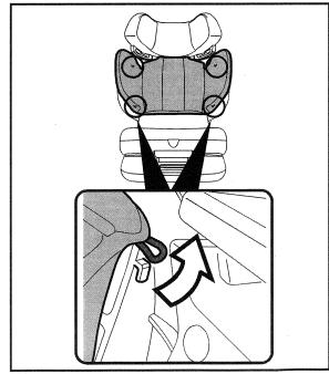
7. Remove the two flaps from their slots on the upper part of the backrest. To help with this operation, raise the headrest. At this point you can remove the lining from the car seat upholstery backrest.
