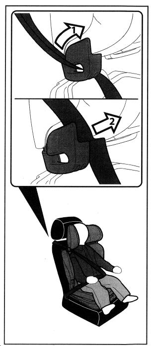
With the child in the booster seat, adjust headrest and backrest height using the levers located behind the seat (refer to pages 13-14). The headrest is properly set when the shoulder belt router is located at no more than 1" (2,5 cm) above shoulder level and the shoulder lies at the center of child's chest.
