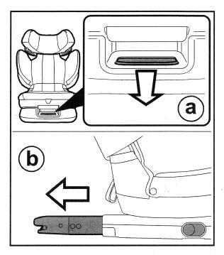
**2.** Attach the connectors to the vehicle seat anchors, ensuring they "click" into place.
